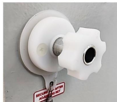
Pull knob out to disengaged RET for tilt adjustment
