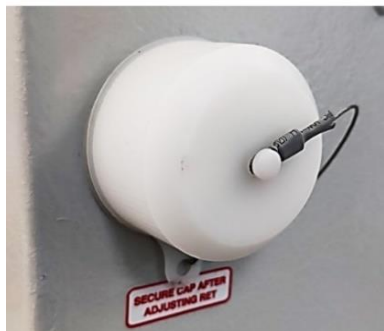
Unscrew/Screw the cap for tilt adjustment process
