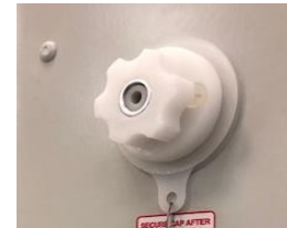
Unscrew/ Screw the cap for tilt adjustment process
