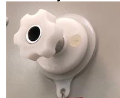
Pull knob out to disengaged RET for tilt adjustment
