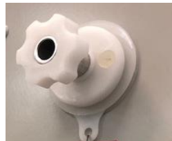
3. Pull knob out to disengaged RET for tilt adjustment
