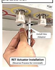
Step 6: RET Actuator Tighten to RET attachment interface
