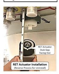
Step 3: Install the Hex adaptor and screw it on
