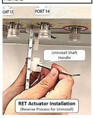
Step 5: RET Actuator stub gap facing out
