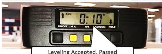
ANTENNA LEVELING ACCEPTED
