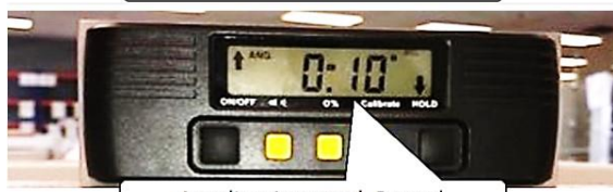
ANTENNA LEVELING ACCEPTED
