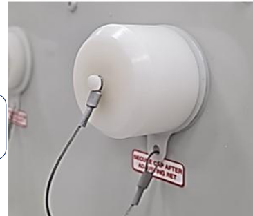
Unscrew/Screw the cap for tilt adjustment process
