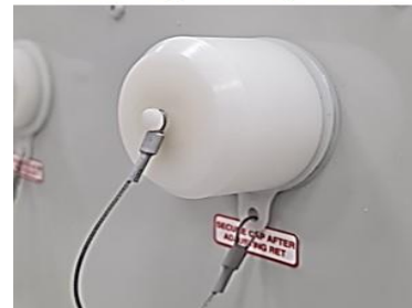
Unscrew/Screw the cap for tilt adjustment process
