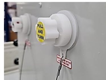
Engaged with internal RET motor position
