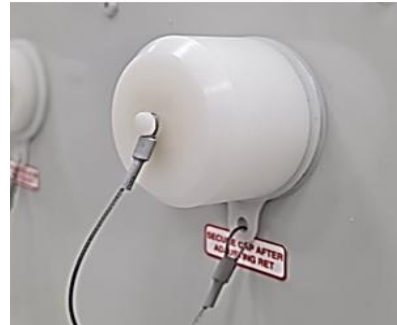
Unscrew/Screw the cap for tilt adjustment process
