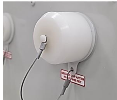
Unscrew/Screw the cap for tilt adjustment process
