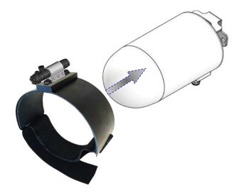
Loosen the pole bracket screw and tilt the 2.50 antenna to the target direction with a laser pointer.
