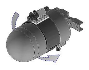
Once position set, tighten the pole bracket 2.60 screw and loosen the Velcro belt to remove the mounting bracket.
